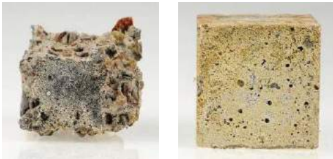
Treated concrete core resists 31% HCL Acid
